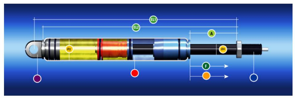
Main type P: Rigid locking in push-in direction, push-out direction relatively rigid
